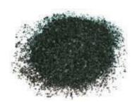
Coconut Shell Activated Carbon 0.55 - 0.75mm
